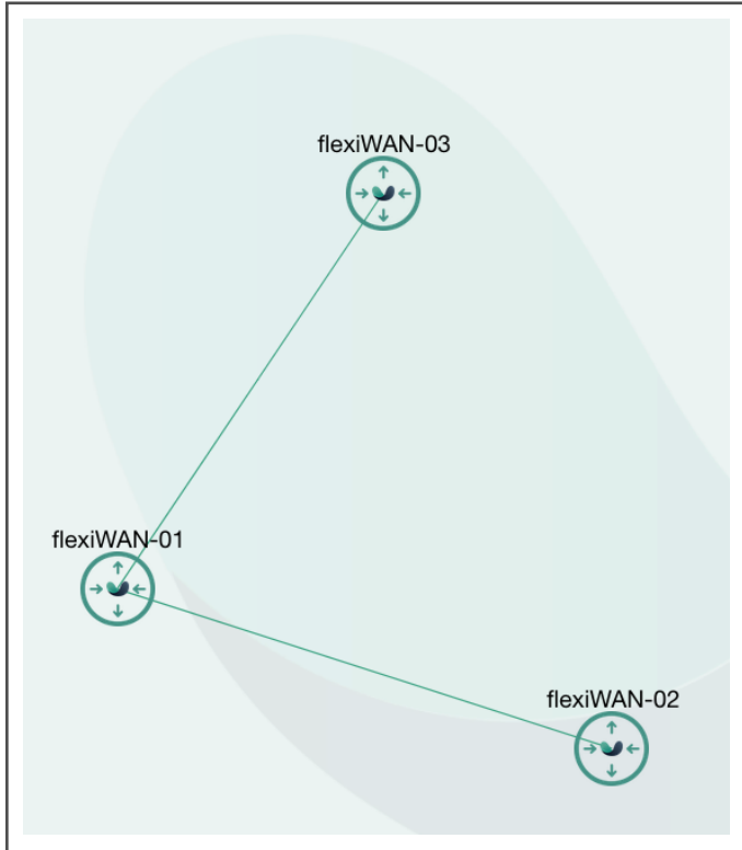
Figure 2. Illustration of the hub-and-spoke network design used in the tests.
